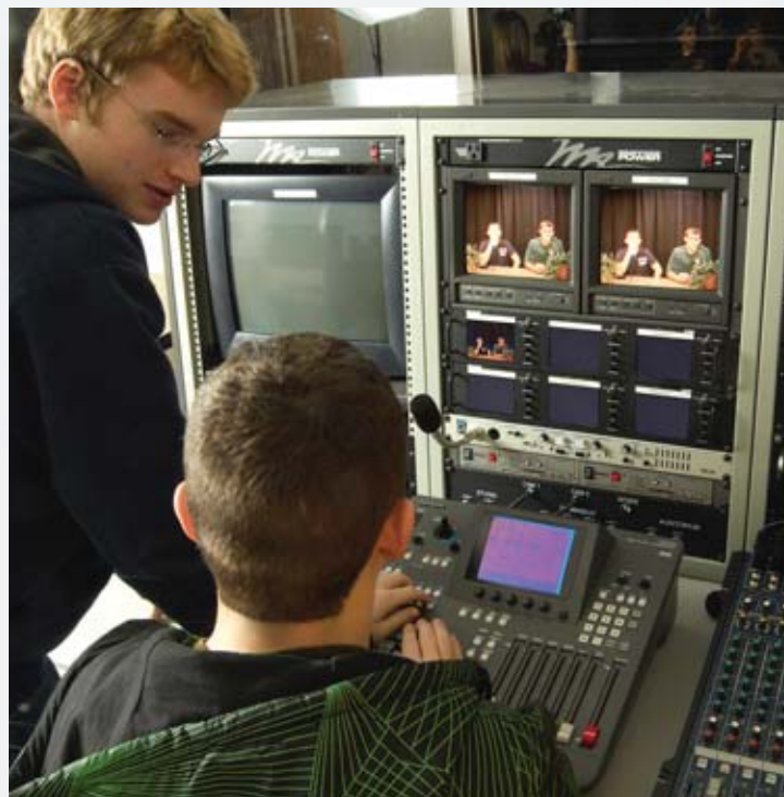
Students at work in the broadcast studio. A VSI encoder built into this production console allows streaming of finished video throughout the school or capture on the eVideon video-on-demand server.
