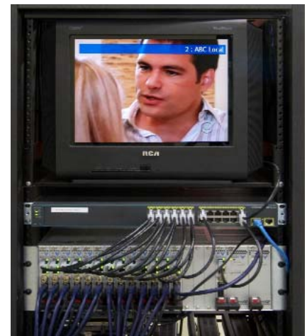
VSI Media Processing Platform at Metro (the system includes four platforms with 57 AVN-220 encoder blades installed)
