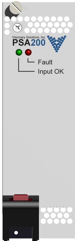
Two LEDs are provided on the PSA200:
