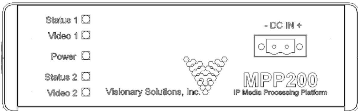
**Status 1** – Copies the status LED pattern of the blade inserted into Slot 1. For more information about the blade, refer to the VSI User's Manual for that blade.
